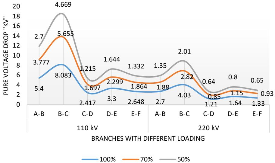
Figure 4: Voltage profile comparison with the 110 kV and 220 kV (Voltage level reduction indicator in case of voltage of 220 kV)
