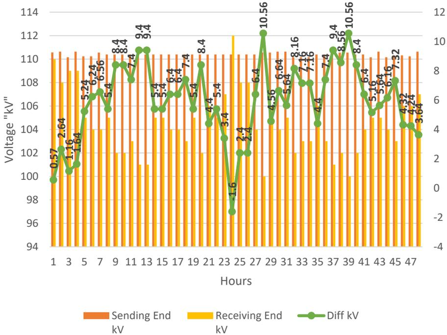
Figure 3: The sending and receiving end voltage profile (source: DABS)
